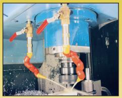
**QPM Check Valves** dramatically speed up coolant response time in this machining center application.
