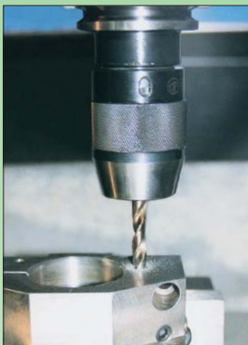
1 Drill coolant passage, leaving reaming allowance.
