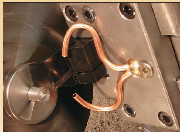
TwinPop nozzle shown installed in lathe turret.
