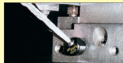
TurretJet shown installed in lathe turret.
