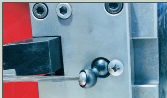
BugEye shown installed on CNC turning center.
