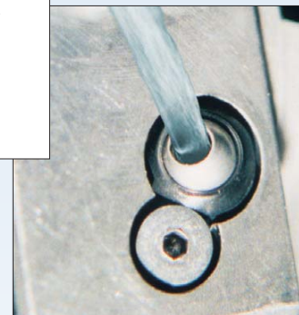
BlackEye installed on quick change turning tool.
