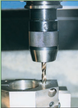
1 Drill coolant passage, leaving reaming allowance.
